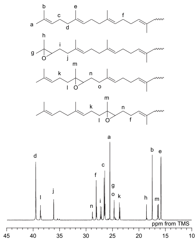
Fig. 13. Expanded ^{13}\text{C} NMR spectrum for partially epoxidized squalene.
